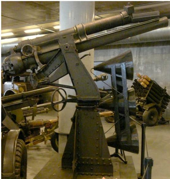
**Ordnance QF 13-pounder 9 cwt; to the immediate right of the pedestal mounting is a listening device with four wooden cones used to detect approaching aircraft and provide information to the gun detachment**
