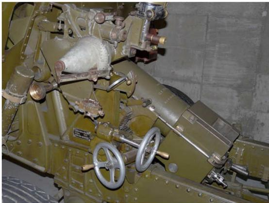
**Ordnance QF 25-pounder Gun Mark II. The dial sight, gun rule, traversing and elevating hand wheels are visible.**
