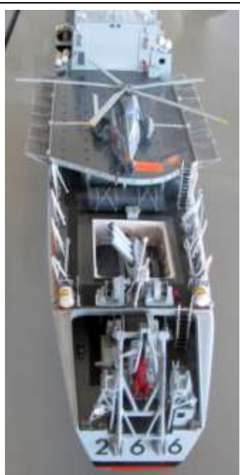
Stern of the CWM model of HMCS Nipigon showing the SQS 504 sonar (the orange body). The boom bobbing gear designed to reduce the impact of pitch and heave on the towed body and the reel of cable attaching it to the ship is shown along with the Sea King helicopter and the Limbo Mortar
