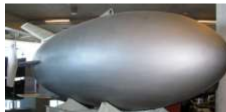
SQA 502 VDS body housing the SQS 505 sonar on the DDH 280 destroyers and Improved Restigouche class frigates.
