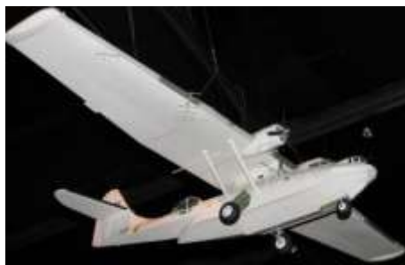
Figure 7: An RCAF Canso flying boat. Typically armed with aircraft depth bombs, it was the most common RCAF ASW aircraft of WWII. It was manufactured in Canada under licence.
